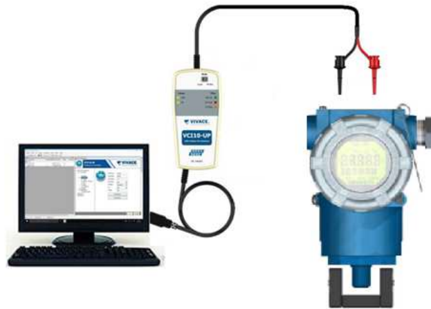
Figure 3.5 – VTP10-P configuration diagram with VCI10-UP.
